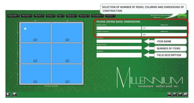
After defining a number of rows, columns and dimensions of construction you should select 'Check'. This function checks whether the construction is possible to be done. If not, Millennium eco Calculator displays a message in red colour including the reasons and returns to previous settings.
